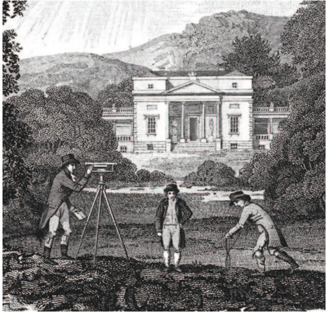
A land surveyor at work, attended by chainmen from John Hampton, architect and land surveyor's business card (c.1810) (National Library of Ireland)
