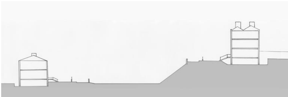
9 – Section through Willow Bank, Vesey Gardens and Vesey Place, showing drop in level between Vesey Place terrace and Willow Bank (drawing by the author)
