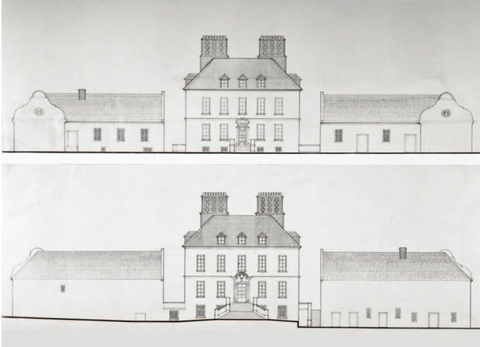
11 – Elevations of the entrance and garden front at Shannongrove, county Limerick, 1709-20 L-shaped service pavilions extend the horizontal emphasis of the main house. (courtesy Irish Architectural Archive)
