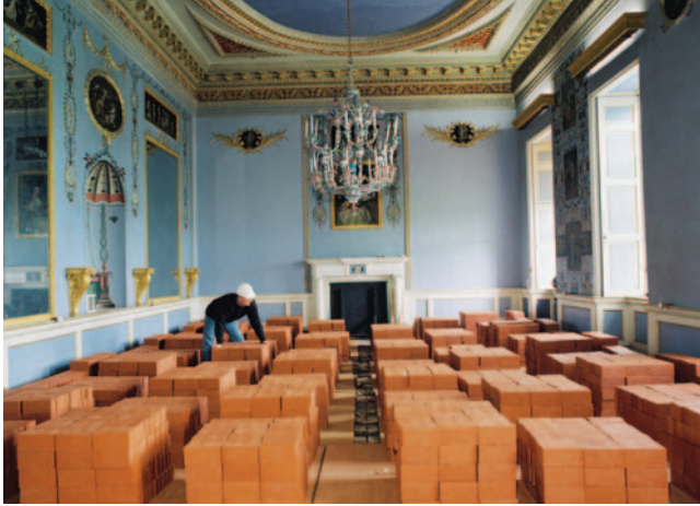
2 – Load-testing in the Long Gallery using bricks (photo: Frank Fennell Photography)
